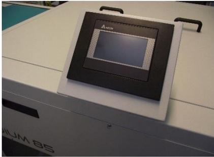
Full Colour LCD Touch Screen HMI Display provides access to all control functions and displays all processing parameters
