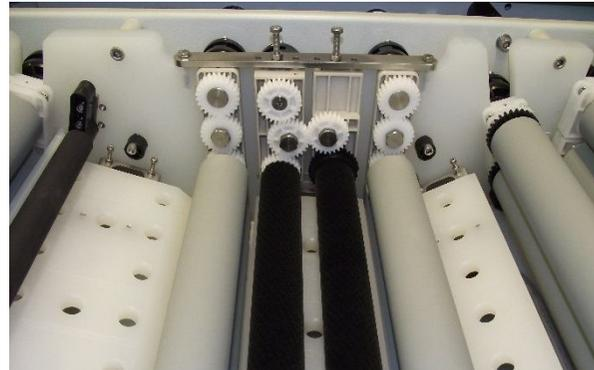
Fully adjustable developer plate guides. Ensures perfect plate alignment into and through the developer section reducing any potential for bow waves
