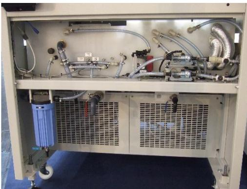
Easy access to all major components including pumps and motors via quick release and removable covers
